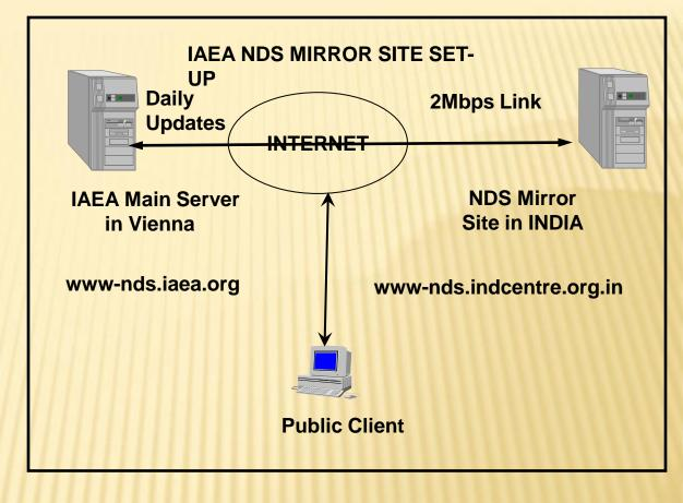
Under this arrangement, online-updating every 12 hours is performed in the mirror with the IAEA website through a 2MB direct link. The server is being maintained by BARC Computer Division - with manpower and machinery. It offers 2-3 times faster downloads in BARC compared to the Vienna site. India offers to collaborate with other network of reaction data centres and help in promoting the online nuclear data services in the coming years. NDPCI Website is under discussion and design stage
